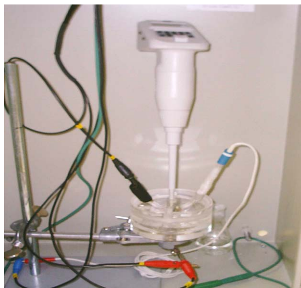
Fig. 1. The detection cell for batch-injection anodic stripping voltammetry with motorized electronic micropipette used for sample injection.
