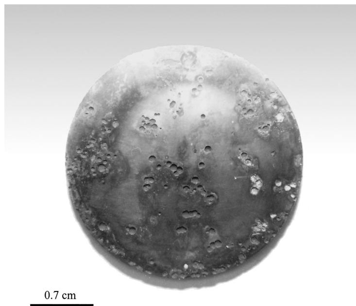
Fig. 2. Optical micrographs of one of the corroded faces of sample Type 3 after removal of the corrosion products.
