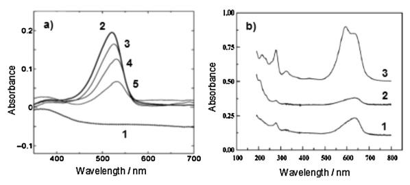
Fig. 17. Absorption spectra of (a) a-SWCNT suspension solution, b-PS solution and c-e-PS/SWCNT: c-10, d-25, and e-50 µg SWCNT: from [95], reproduced by permission of Elsevier; (b) a-NB monomer, b-NB/SWCNT and c-PNB/SWCNT: from [62], reproduced by permission of Elsevier.
