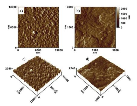
Fig. 15. AFM and 3D images of PNR (a and c) and PNR/MWCNT composite films (b and d). From [7], reproduced by permission of Elsevier.
