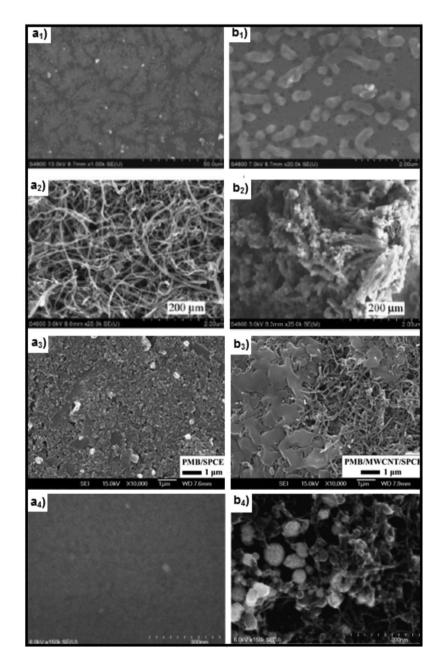
**Fig. 13.** SEM micrographs of (a<sub>1</sub>) SWCNT/PTBO/GCE and (b<sub>1</sub>) magnification of a<sub>1</sub>: from [89], reproduced by permission of Springer; (a<sub>2</sub>) thin and (b<sub>2</sub>) thick film PTH/MWCNT/ GCE: from [81], reproduced by permission of Wiley; (a<sub>3</sub>) PMB/SPCE and (b<sub>3</sub>) PMB/MWCNT/SPCE: from [45], reproduced by permission of Elsevier; (a<sub>4</sub>) PPS/GCE and (b<sub>4</sub>) PPS/ SWCNT/GCE: from [95], reproduced by permission of Elsevier.
