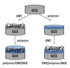
Fig. 1. Schematic preparation of CNT/polymer modified electrodes.
