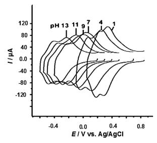
**Fig. 11.** CVs at of PMB/MWCNT/GCE in different pH;  $E_{pa,c}$ (mV) = 203–35 pH and  $E_{1/2}$ (mV) = 400–64 pH. From [49], reproduced by permission of Elsevier.
