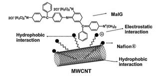
**Fig. 3.** Possible interaction between CNT, Nafion (NF) and MalG. From [41], reproduced by permission of Elsevier.
