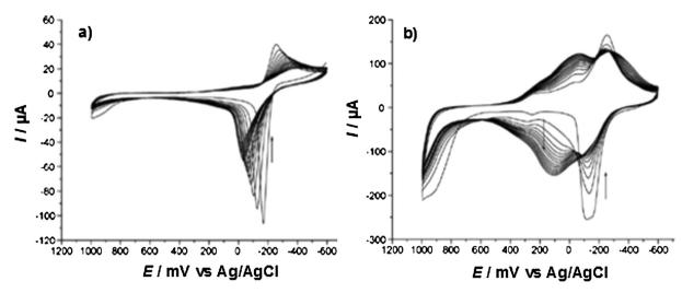
Fig. 8. CVs recorded during polymerization of TBO at (a) MWCNT/GCE and (b) GCE in a solution containing 5 mM TBO in PBS pH 7.4; v = 50 mV s<sup>-1</sup>. From [83], reproduced by permission of Elsevier.
