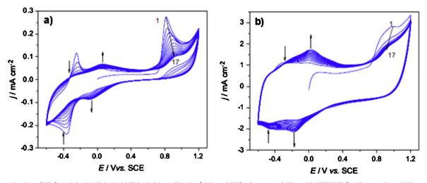
Fig. 6. Polymerization of NB from 0.5 mM NB in 0.1 M PBS pH 6.0;  $v = 50 \text{ mV s}^{-1}$  (A) on GCE for 5 scans and (B) on MWCNT/GCE for 17 scans. From [63], reproduced by permission of Elsevier.
