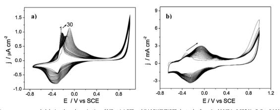
**Fig. 5.** Cyclic voltammograms recorded during the polymerization of MB at (a) CCE and (b) MWCNT/CCE electrodes from 1 mM MB in 0.025  $Na_2B_4O_7$ +0.1 M  $Na_2SO_4$  pH 9.2; v = 50 mV s<sup>-1</sup>. From [50], reproduced by permission of Wiley.
