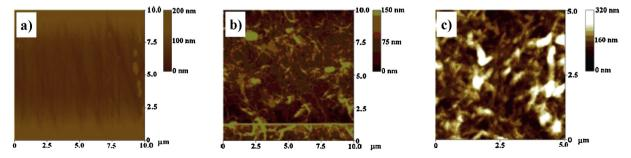
Fig. 16. AFM images of (a) PBCB/GCE, (b) SWCNT/GCE and (c) PBCB/SWCNT/GCE. From [30], reproduced by permission of Elsevier.
