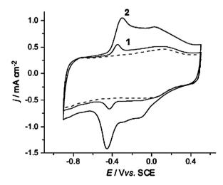
**Fig. 9.** Cyclic voltammograms at MWCNT/GCE (dashed line) and (a) MWCNT/PNB/ GCE and (b) PNB/MWCNT/GCE;  $v = 25 \text{ mV s}^{-1}$ . From [63], reproduced by permission of Elsevier.
