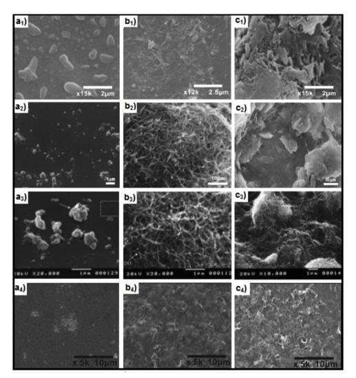
**Fig. 14.** SEM images of ITO electrodes modified with  $(a_1)$  PMalG,  $(b_1)$  MWCNT,  $(c_1)$  MWCNT/PMalG: from [41], reproduced by permission of Elsevier;  $(a_2)$  PBG,  $(b_2)$  MWCNT,  $(c_2)$  PBG/MWCNT: from [38], reproduced by permission of Springer;  $(a_3)$  PNR,  $(b_3)$  MWCNT,  $(c_3)$  PNR/MWCNT: from [72], reproduced by permission of Springer;  $(a_4)$  PBCB,  $(b_4)$  MWCNT and  $(c_4)$  PBCB/MWCNT: from [36], reproduced by permission of The Electrochemical Society.
