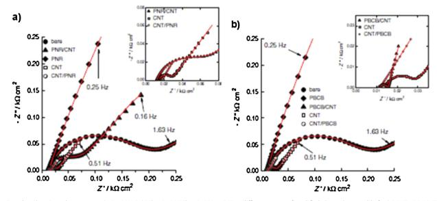
**Fig. 12.** Complex plane impedance spectra in 3 mM K<sub>3</sub>Fe(CN)<sub>6</sub> + 0.1 M KCl at 0.15 V vs. SCE at different stages of modified electrode assembly for (a) PNR + MWCNT and (b) PBCB + MWCNT modified electrodes. The magnified insets show the spectra of only MWCNT and their combination with polymers. Lines show equivalent circuit fitting. From [31], reproduced by permission of Springer.
