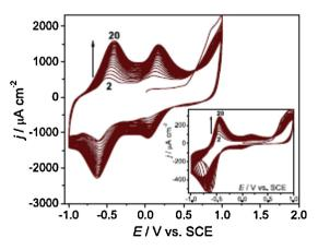
**Fig. 7.** CVs recorded during polymerization of NR at MWCNT/GCE in 1 mM NR + 0.025 M KPB + 0.1 M KNO3 (pH 5.5) from -1.0 to + 1.0 V vs. SCE at 50 mV s<sup>-1</sup>; in inset polymerization at bare GCE. From [31], reproduced by permission of Springer.
