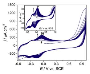
**Fig. 4.** Polymerization of BCB at MWCNT/GCE and GCE in inset from 0.1 mM BCB in 0.1 M PBS pH 7.0+0.1 M KNO<sub>3</sub>. From [31], reproduced by permission of Springer.
