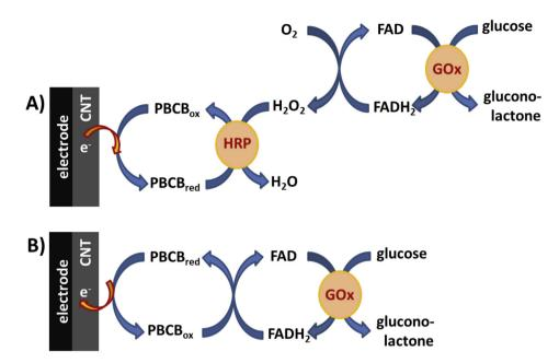
**Fig. 18.** GOx biosensor mechanism (A) in a bi-enzymatic configuration, when detection is based on the detection of peroxide formed in the first GOx enzymatic reaction and (B) based on the direct regeneration of FAD at polyphenazine mediator.
