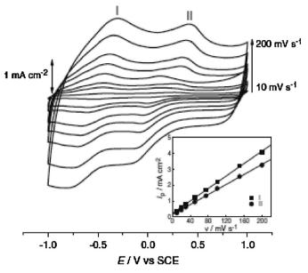
**Fig. 10.** CVs at PNR/MWCNT/GCE at different scan rates, v, between 10 and 200 mV s<sup>-1</sup>; the inset is the plot of the anodic peak currents (I) and (II) vs. v. From [72], reproduced by permission of Springer.
