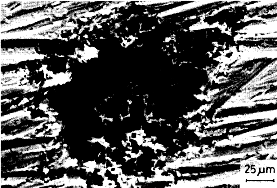
FIG. 7. Scanning electron micrograph showing pit formation after exposure for 20 min at -0.5 V(SCE) in a solution containing 0.10 M \text{NaNO}_2 + 0.10 M \text{KCl} + 0.33 M \text{K}_2\text{SO}_4 .
