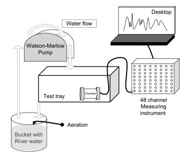
Fig. 1. Experimental setup: MFB (chambers, measuring instrument and desktop), bucket with aeration and peristaltic pump.
